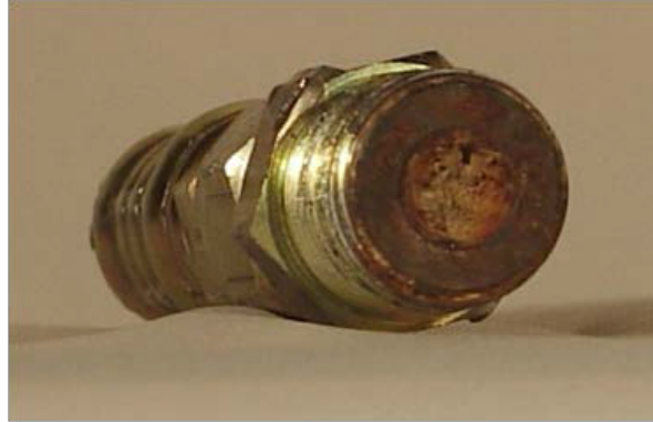
Figure 2. Plugged extruder \frac{3}{8} inch zone inlet coupling.
