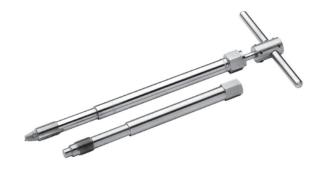
This cleaning tool kit provides two tools to remove excess plastic from transducer mounting holes, prior to installation. Installation of transducers into plugged and/or dirty mounting holes is a major cause of installation related damage. The cleaning tool is to be used when the polymer is molten. Comes in storage case with instructions.
